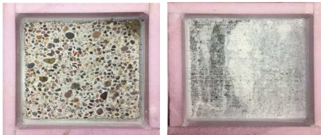
Control sample without PAVIX and curing compound Sample with PAVIX and curing compound
