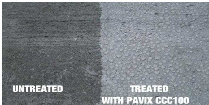
Fig. 1: Water contact angles ( \theta ) for concrete surfaces comparing control (left) & Pavix-treated (right) using TX-DOT pavement mix design at w/c=0.47
